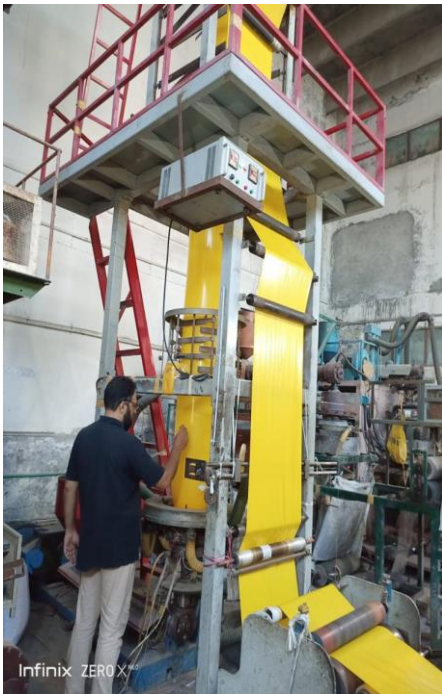
Extrusion machine used to melt plastic granules and give them a sheet like look
