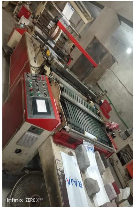
Machine that cuts plastic sheet according to required size
